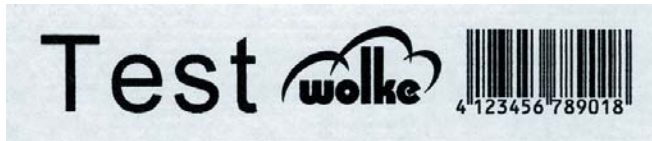
Fig. 7_183: Printing Example with 2 Nozzle Rows = 600dpi
