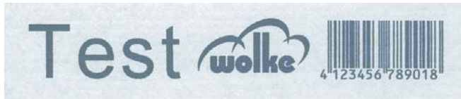
Fig. 7_182: Printing Example with 1 Nozzle Row = 300dpi
